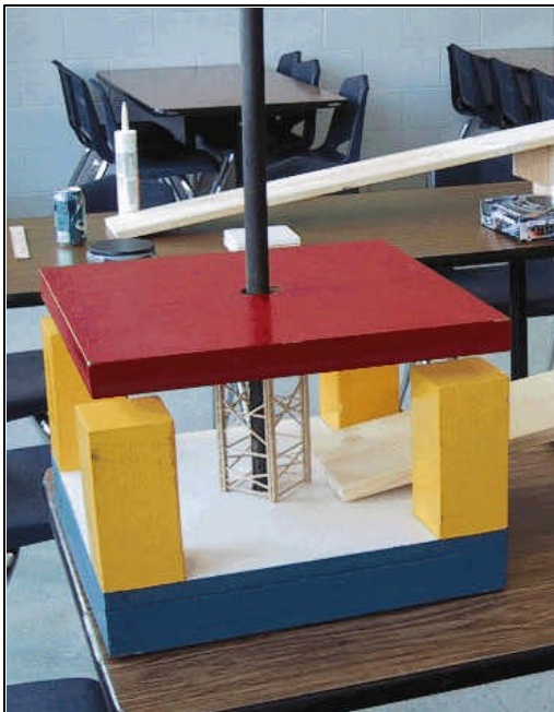
An Odyssey of the Mind “Crusher” or Structure Tester. The ramp at the right was used in the 2000-2001 Balsa Long-Term Problem and is not part of the normal Structure Tester in most years.
